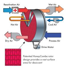
In the 1950's Munters invented modern industrial dehumidification when it introduced the self-regenerating desiccant rotor, the heart of the dehumidifier.
